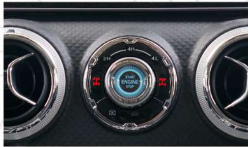
ELECTRONIC SELECTABLE 4X4 DRIVE MODES BY BORGWARNER SYSTEM
